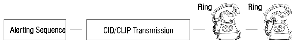
Figure 32. Type I - CID or CLIP Sequence of Events
